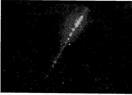
Fig. 3. - A track photographed, in the electric field direction, with the image intensifier.
